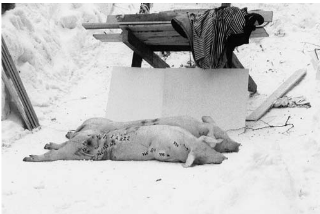
Fig. 5 Position of the two swine when three gunshot hits were inflicted through them both sequentially
